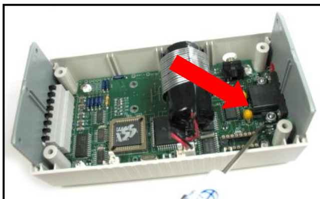
Dielectric Insert for Line-Powered ELITEpros
