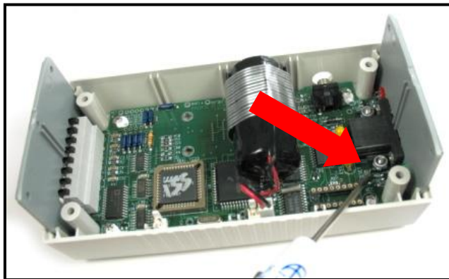
DATApr RESET and GND Pins
